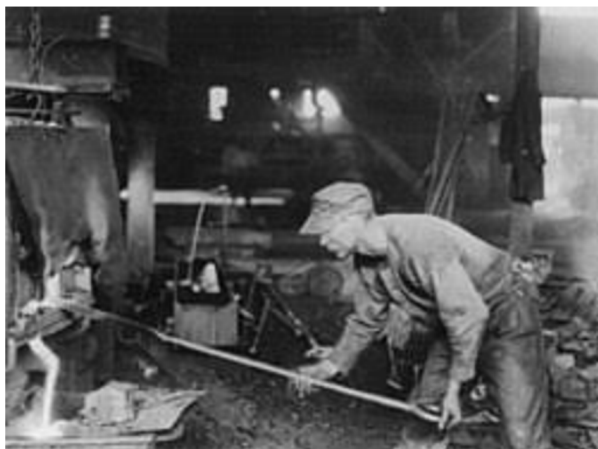
A puddler draining steel from a furnace to create a ball of molten iron, which he will carry to the rolling mill to be fabricated into useful steel items.
