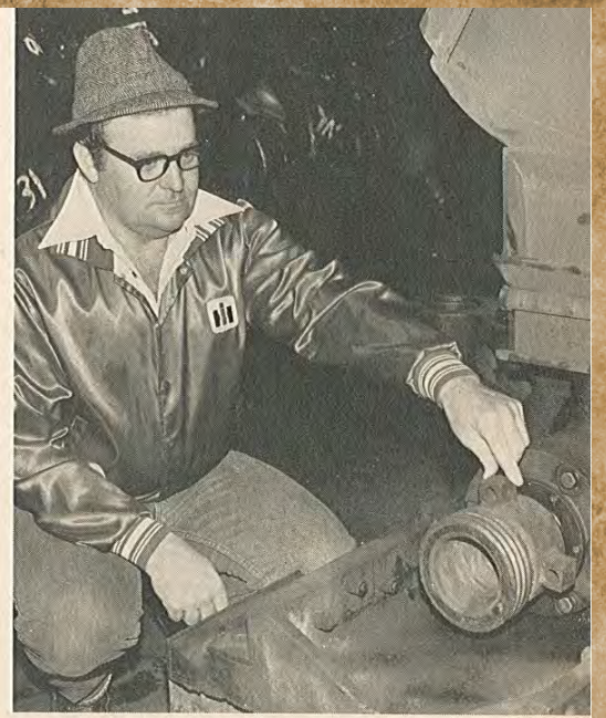
The Third Award in the Employee Suggestion Plan was earned by Richard W. Clapper, elongator operator - Number Four Tube Mill - Gambrinus Steel Plant. He received 45 shares of stock for his idea to use a left-hand threaded retaining nut to secure the mandrel bar on the Number Four Piercing Mill. Clapper's suggestion improved productivity and quality.
